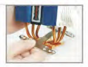
Place the heat sink on the CPU core.
